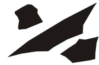
**Sub-Angular/ Rounded:** particles show definite to considerable wear; the edges and corners are rounded sometimes to smooth curves.
