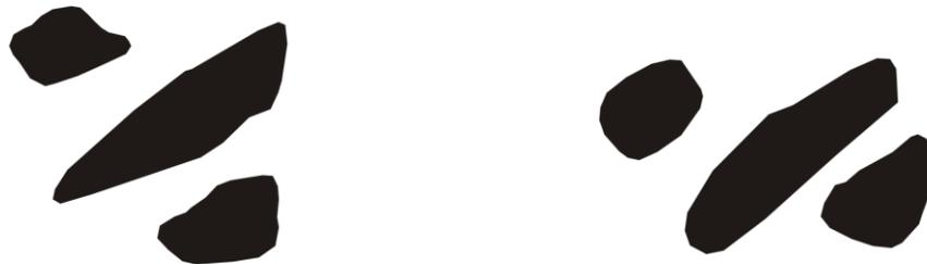
**Rounded:** Most surfaces of the particle show considerable wear. Edges and corners are reduced to broad curves.
