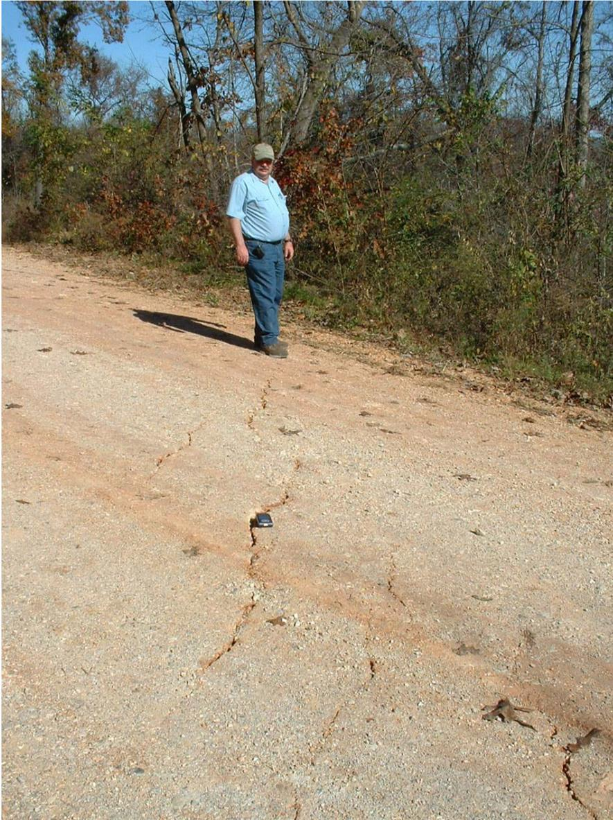
Sub-parallel tension cracks, slight down slope offset to the southeast, trending N130°W, near crest of rise, northeast edge of slide area, Blackjack Lane. Latitude 36.18281, Longitude: -93.19977.
