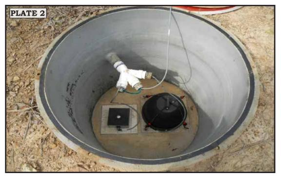
Accelerometer (left) and broadband seismometer with protective igloo cover
