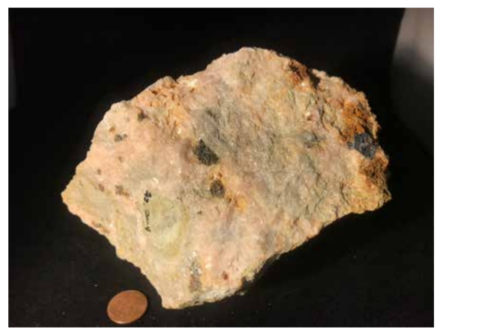
Dolomite, Sphalerite, and Galena in brecciated dolomite of the Everton Formation. Golconda Prospect.
