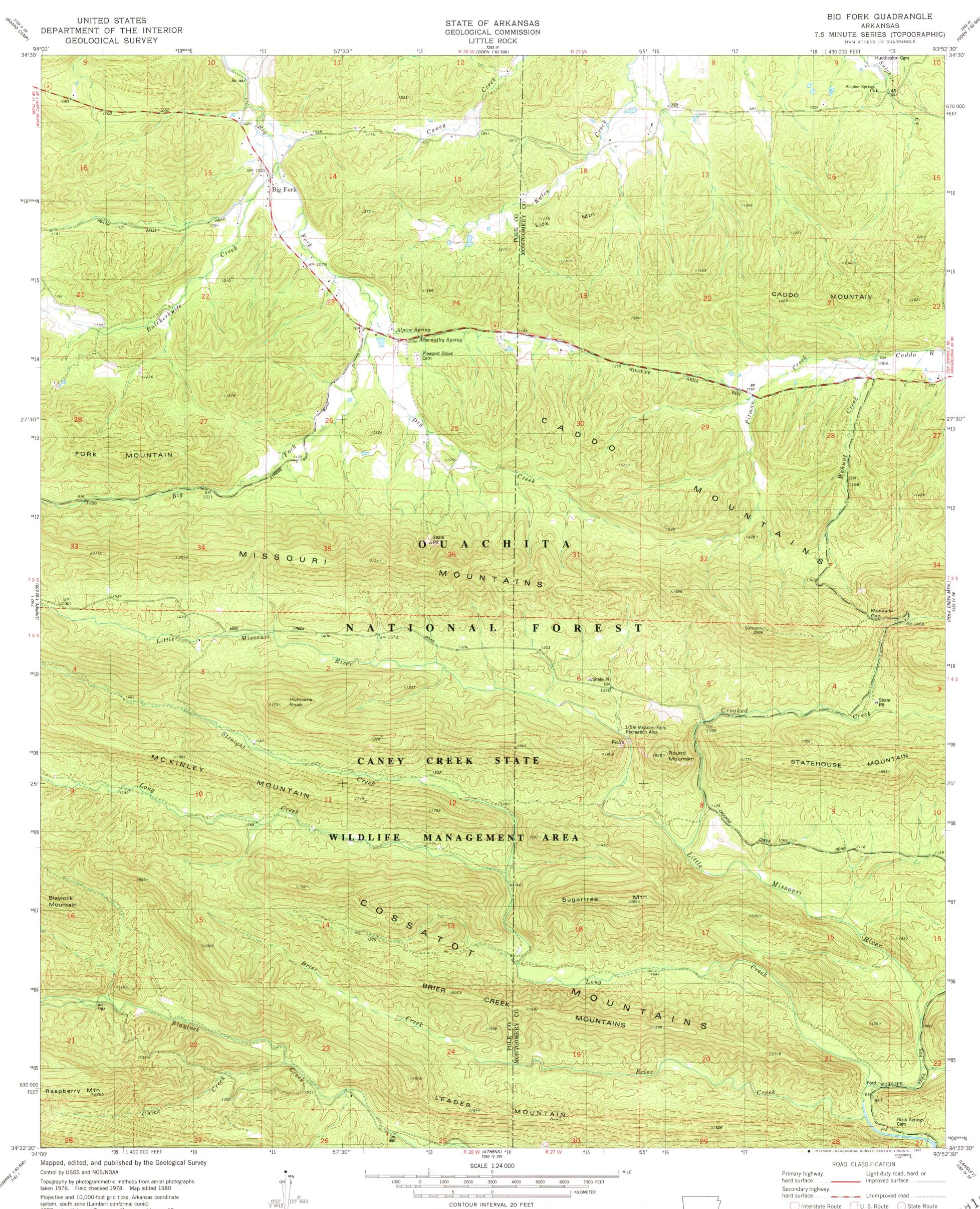
system, south zone (Lambert conformal conic) 1000-meter Universal Transverse Mercator grid, zone 15 1927 North American Datum To place on the predicted North American Datum 1983 move the projection lines 7 meters south and 18 meters east as shown by dashed corner ticks
