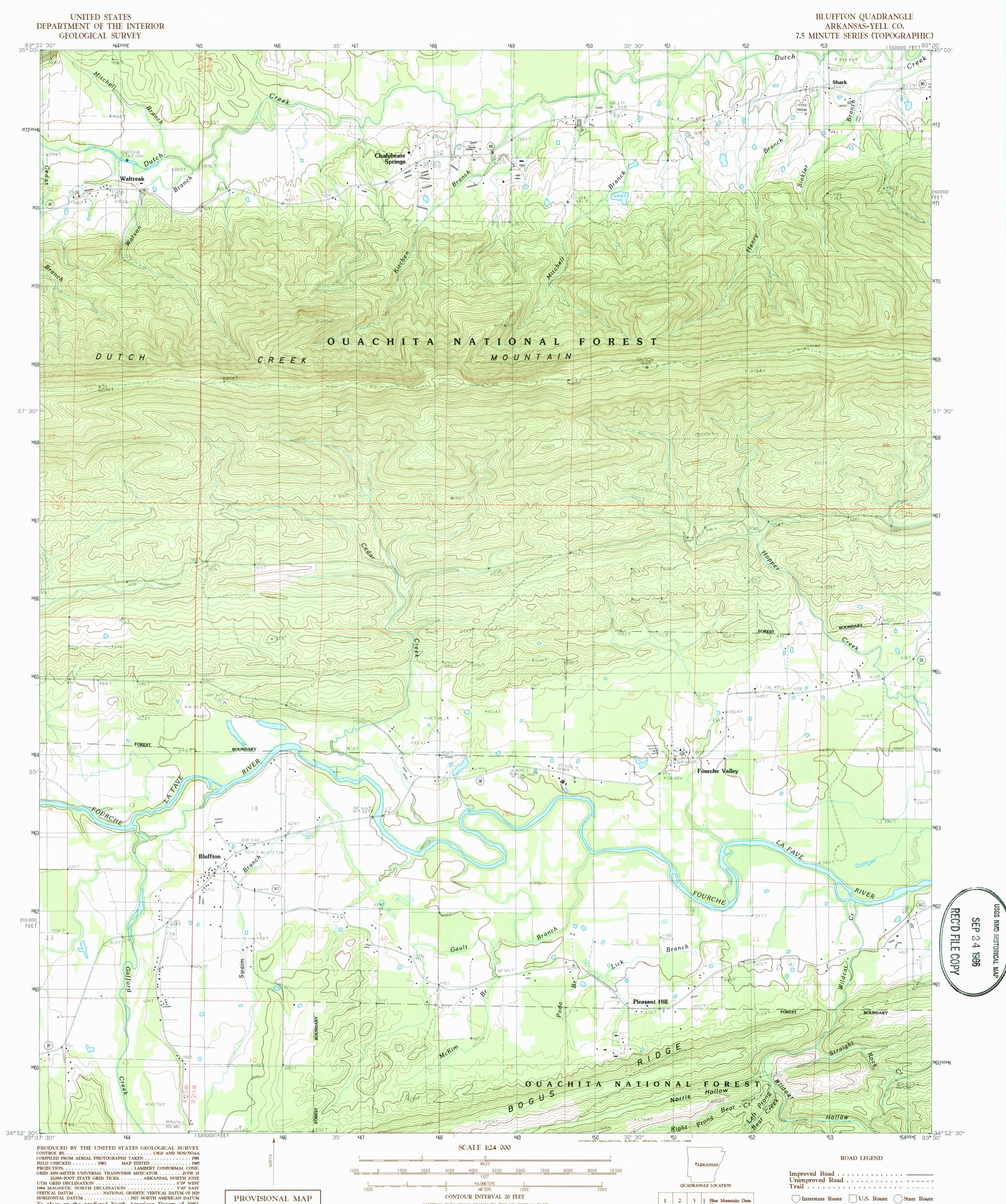
To place on the predicted North American Datum of 1983, move the projection lines as shown by dashed corner ticks (7 meters south and 17 meters east) There may be private inholdings within the boundaries of any Federal and State Reservations shown on this map No distinction made between houses, barns, and other buildings
