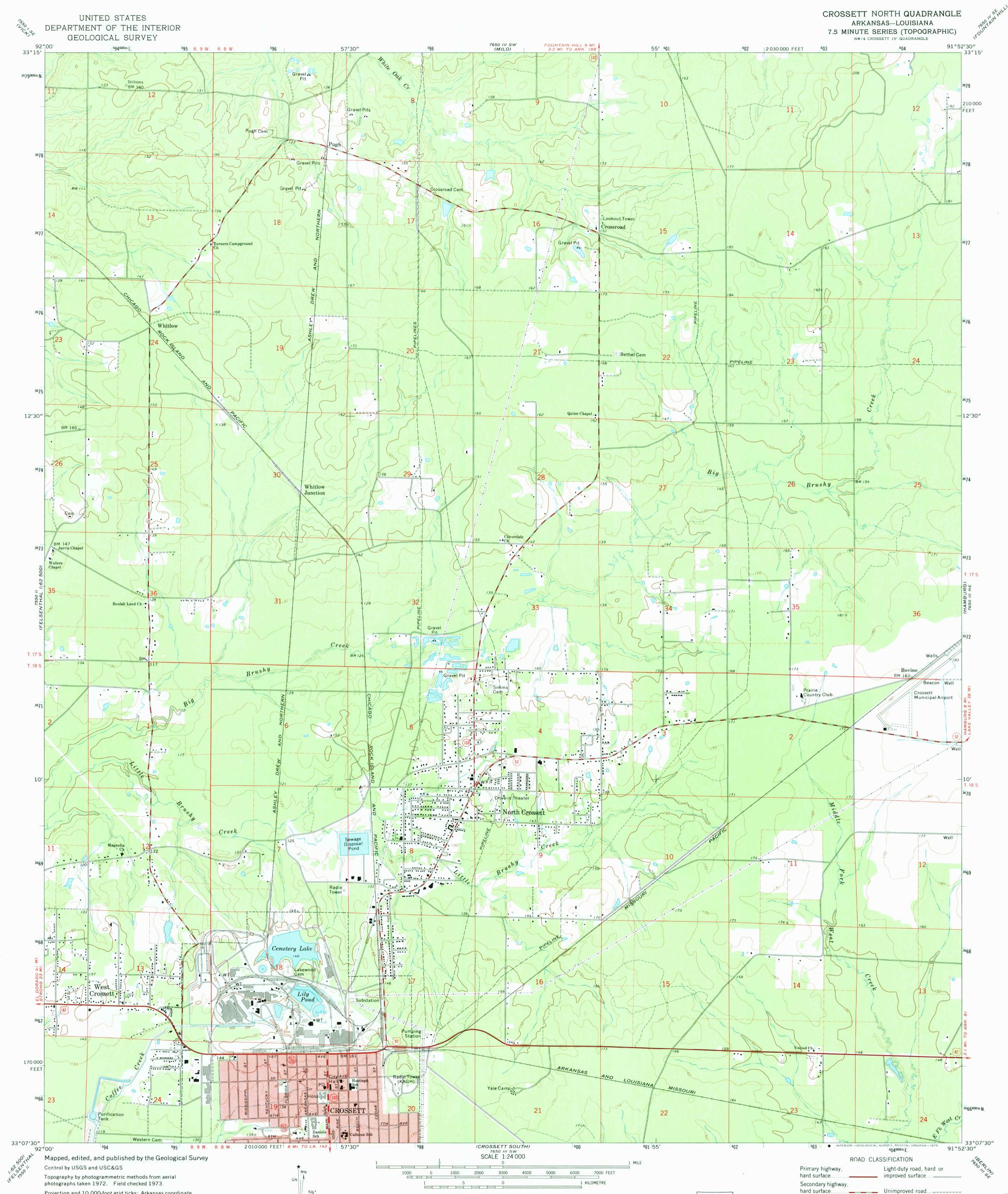
Projection and 10,000-foot grid ticks: Arkansas coordinate system, south zone (Lambert conformal conic) 1000-metre Universal Transverse Mercator grid ticks, zone 15, shown in blue. 1927 North American datum
