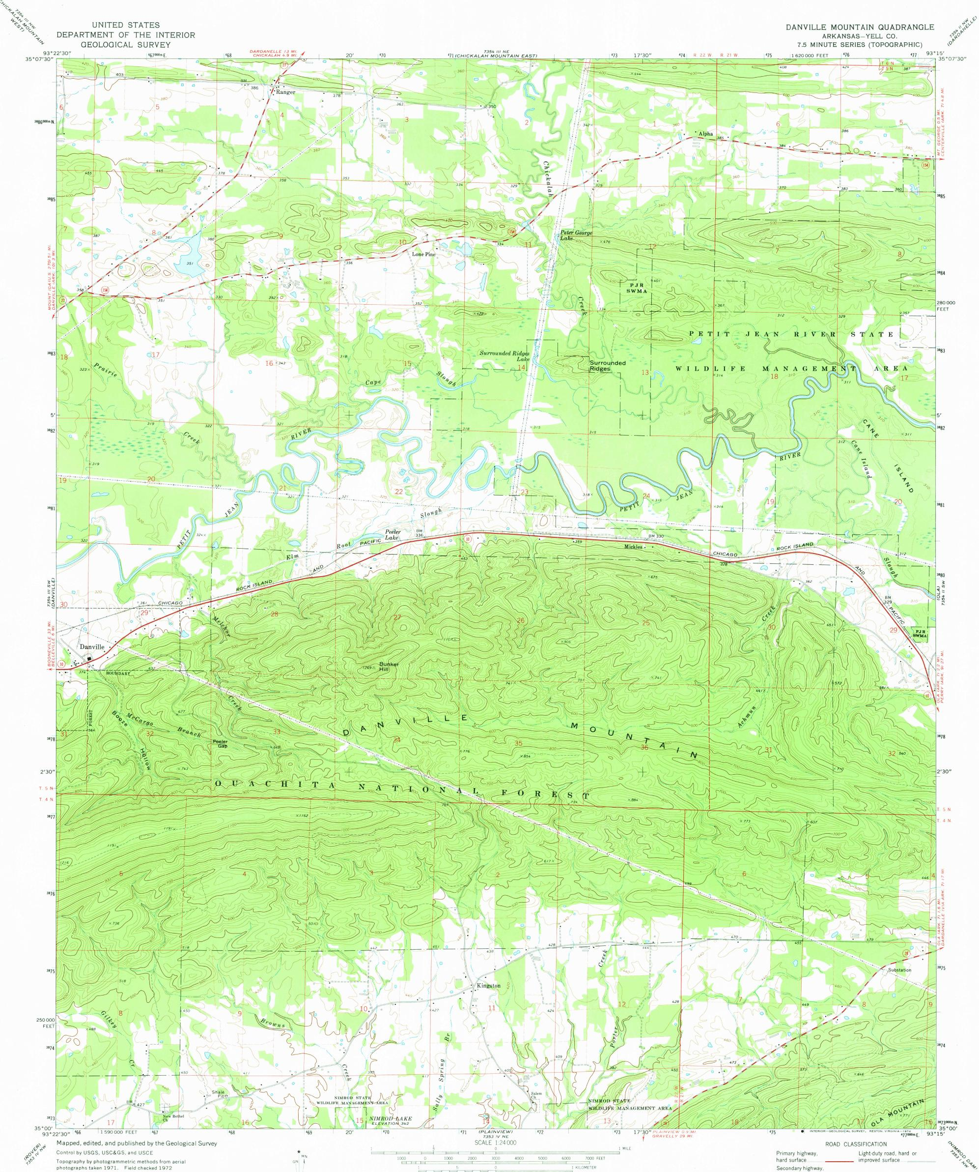
Projection and 10,000-foot grid ticks: Arkansas coordinate system, north zone (Lambert conformal conic) 1000-meter Universal Transverse Mercator grid ticks, zone 15, shown in blue. 1927 North American datum Areas covered by dashed light-blue pattern are subject to controlled inundation to 373 feet
