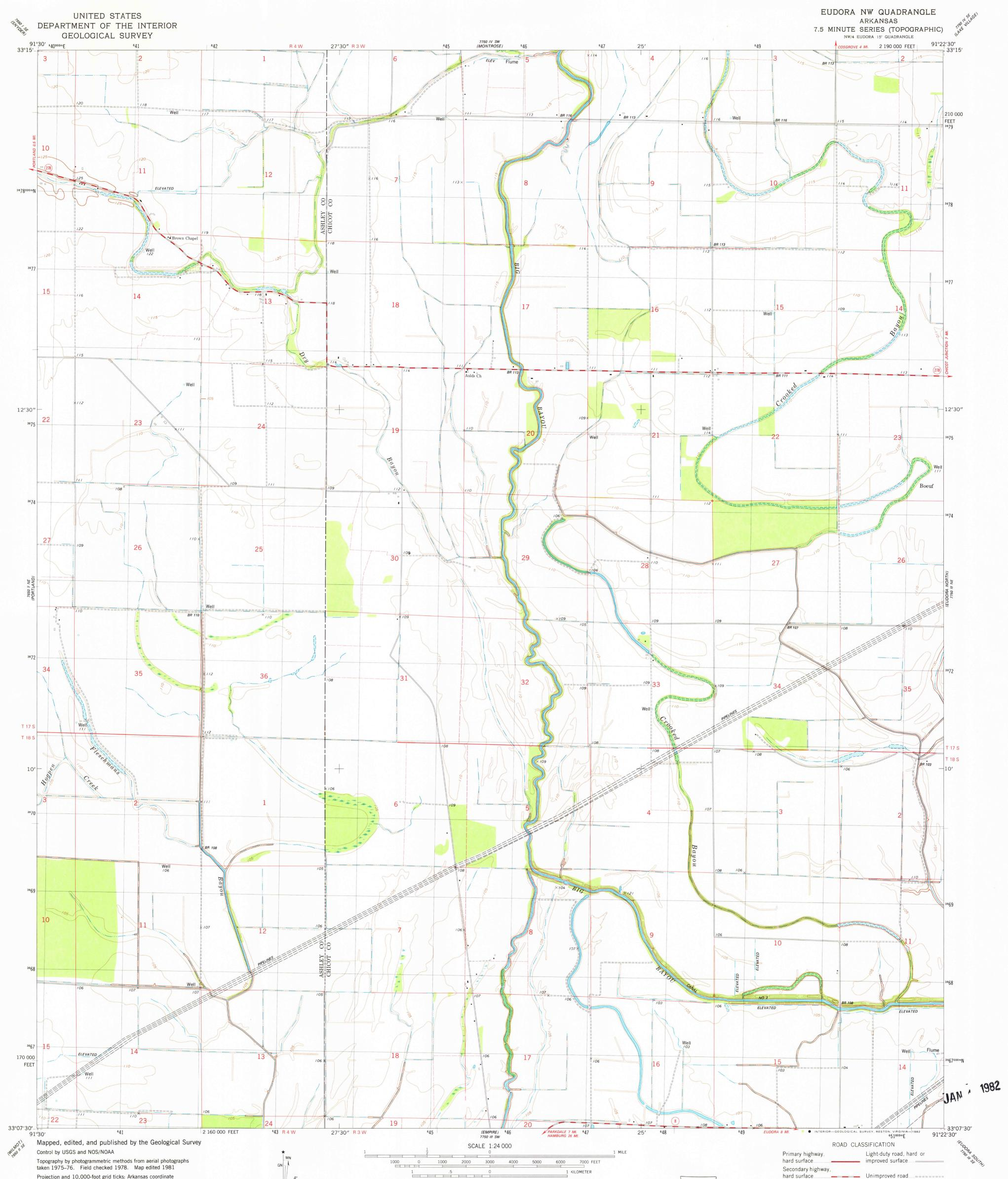
Projection and 10,000-foot grid ticks: Arkansas coordinate system, south zone (Lambert conformal conic) 1000-meter Universal Transverse Mercator grid, zone 15 1927 North American Datum To place on the predicted North American Datum 1983 move the projection lines 11 meters south and 11 meters east as shown by dashed corner ticks
