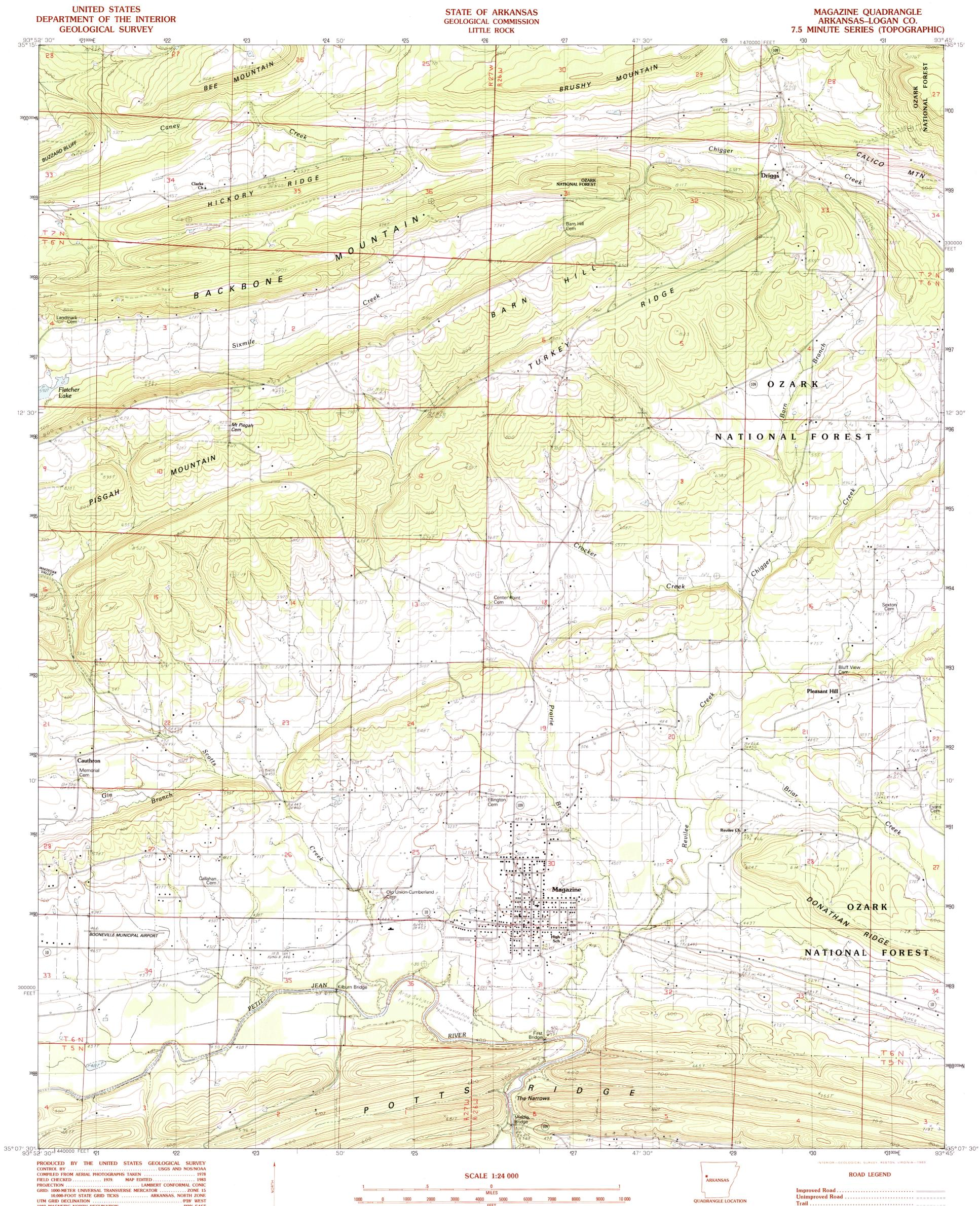
1983 MAGNETIC NORTH DECLINATION . . 5°30' EAST VERTICAL DATUM ...... NATIONAL GEODETIC VERTICAL DATUM OF 1929 HORIZONTAL DATUM .... ..... 1927 NORTH AMERICAN DATUM To place on the predicted North American Datum of 1983 move the projection lines as shown by dashed corner ticks (6 meters south and 17 meters east) There may be private inholdings within the boundaries of any Federal and State reservations shown on this map
