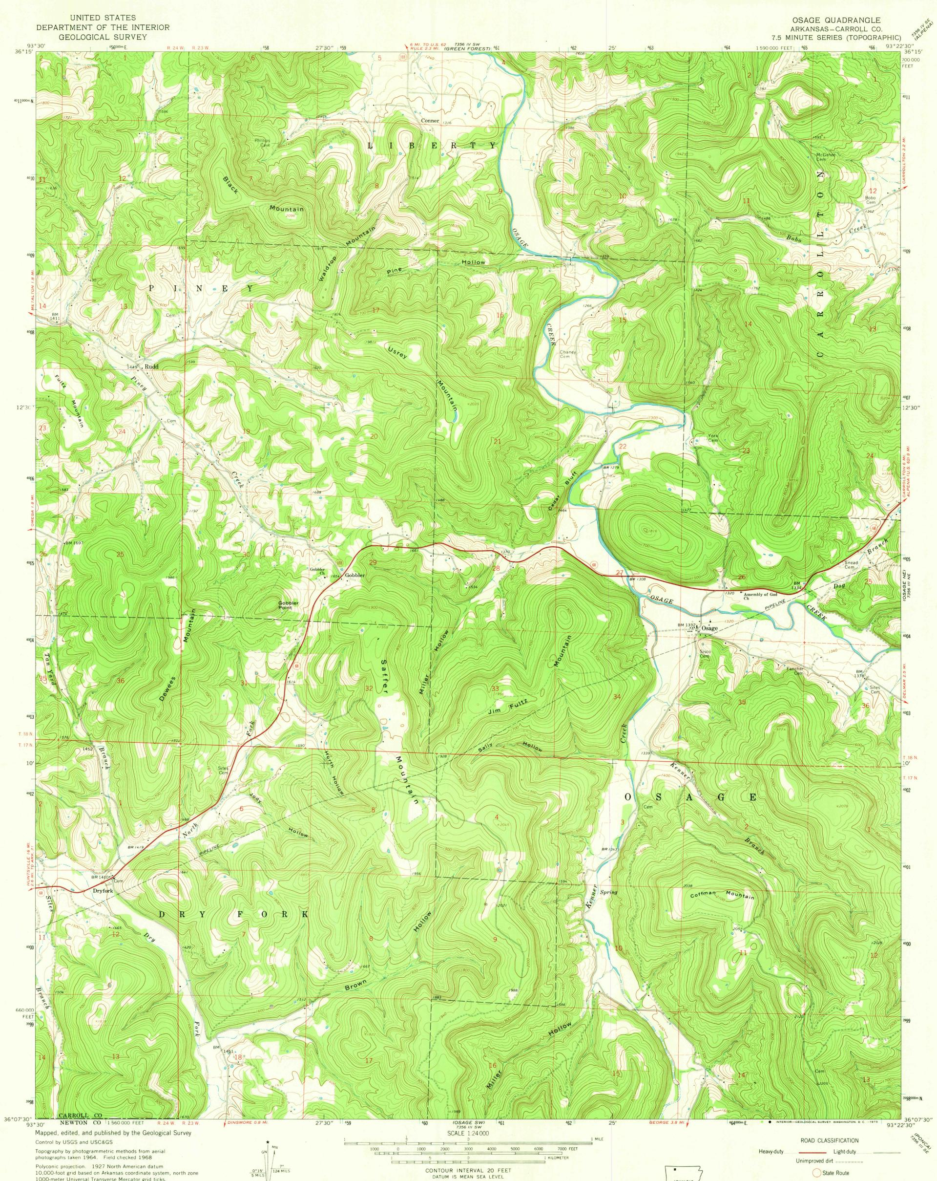
Polyconic projection. 1927 North American datum 10,000-foot grid based on Arkansas coordinate system, north zone 1000-meter Universal Transverse Mercator grid ticks, zone 15, shown in blue
