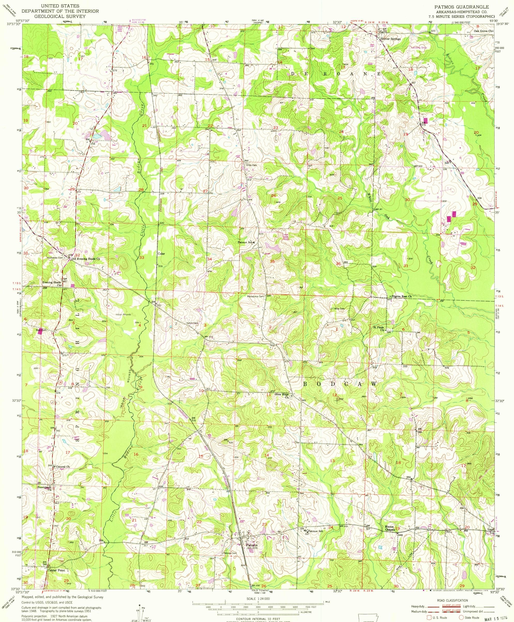
10,000-foot grid based on Arkansas coordinate system, south zone 1000-metre Universal Transverse Mercator grid ticks, zone 15, shown in blue
