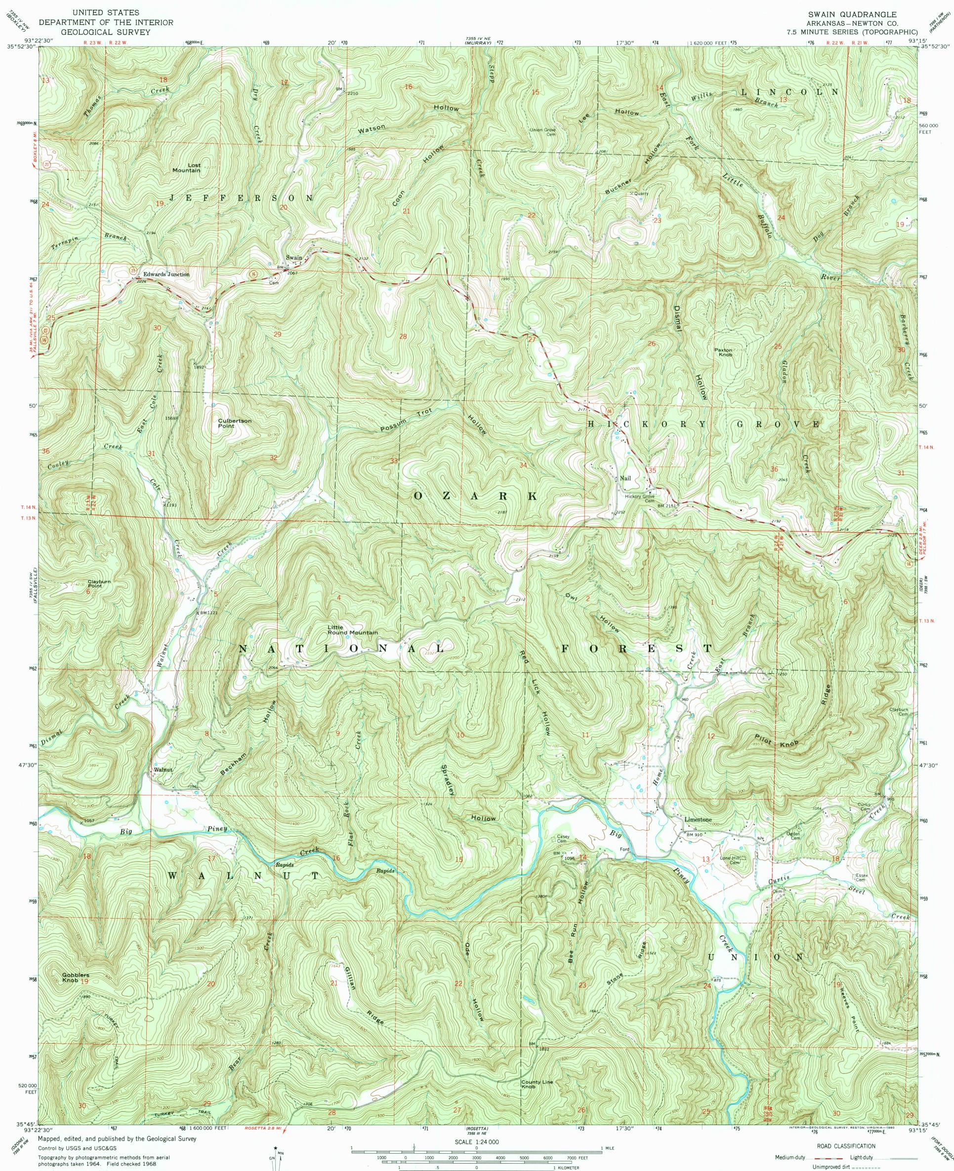
Polyconic projection. 1927 North American datum 10,000-foot grid based on Arkansas coordinate system, north zone CONTOUR INTERVAL 20 FEET
