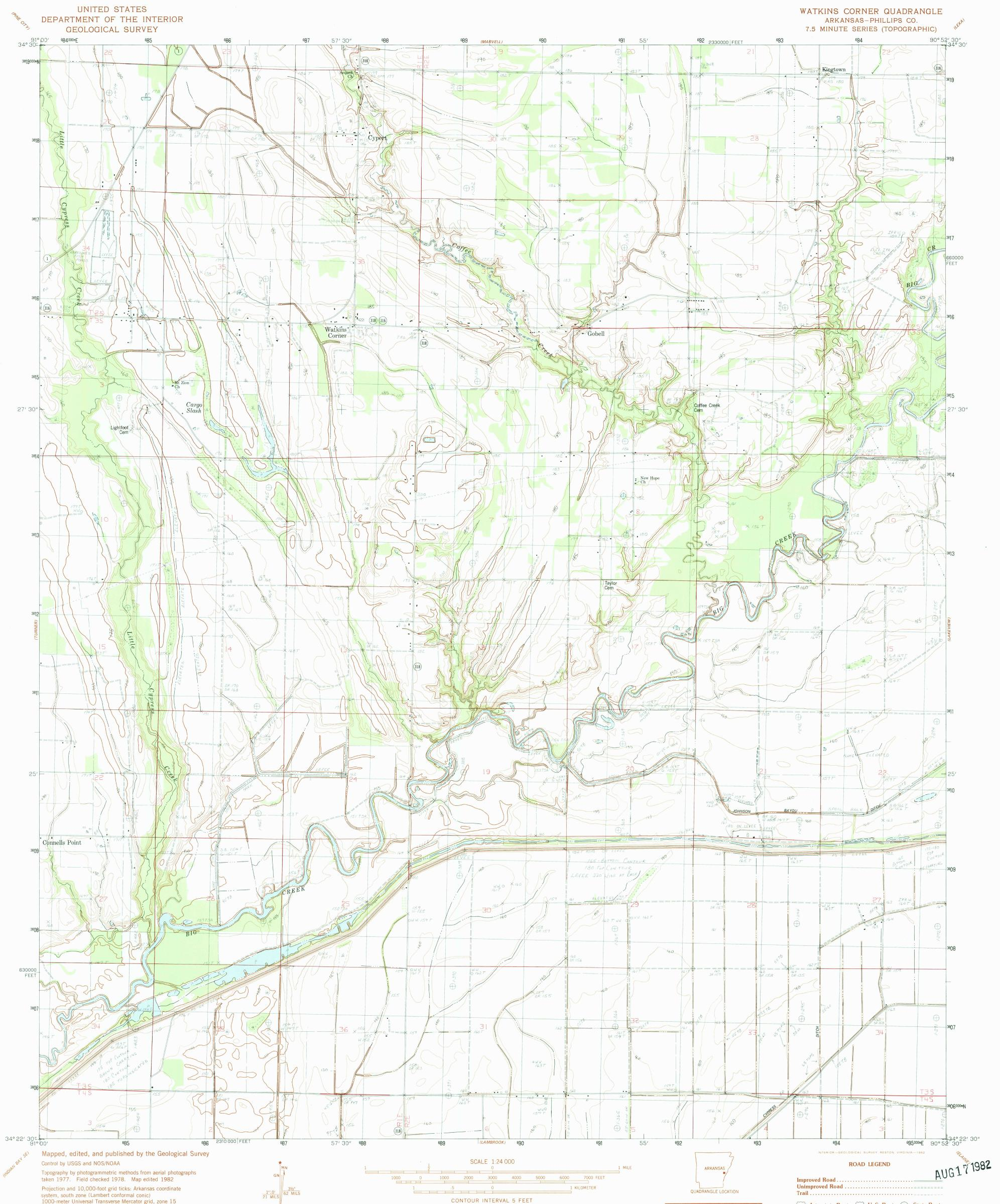
1000-meter Universal Transverse Mercator grid, zone 15 1927 North American Datum To place on the predicted North American Datum 1983 move the projection lines 8 meters south and 10 meters east as shown by dashed corner ticks
