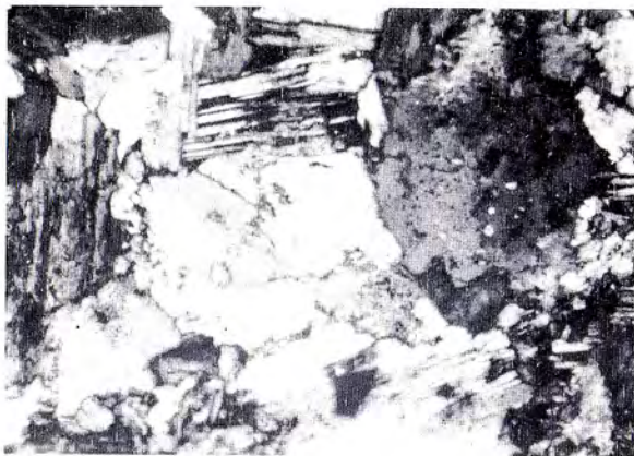
A. Thin section of coarse-grained albite-perthite-carbonate vein, West Pit. All grains are feldspar. Crossed nicols. X 80.
