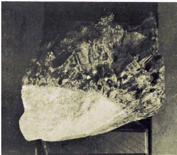
Figure 8. Hand specimen showing smoky quartz vein—gray quartzite contact, Hardy-Walsh brookite deposit. Natural size.
