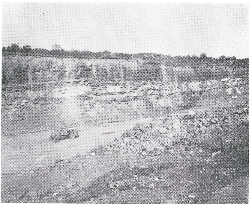
Figure 2. Quarry face of Jackfork Sandstone in Jeffrey quarry (June 1962). Shows well bedded sandstone and shale, and absence of strong folding.
