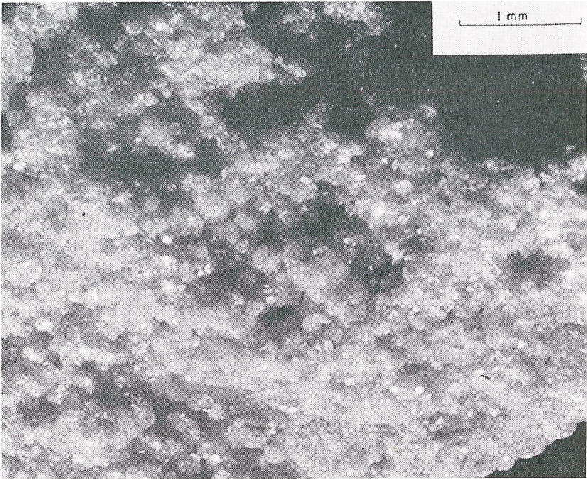
Figure 11. Massive very pure white cookeite aggregate without quartz, Jeffrey quarry (analyzed material).
