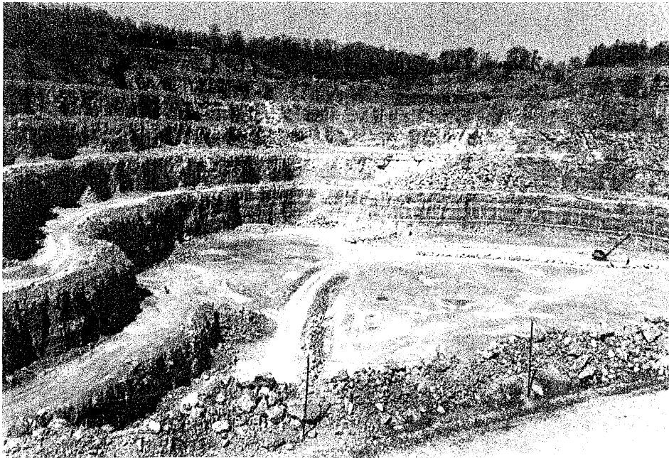
Figure 15. Limestone quarry, Ozark region, Independence County. Benches approximately 40 feet in height.
