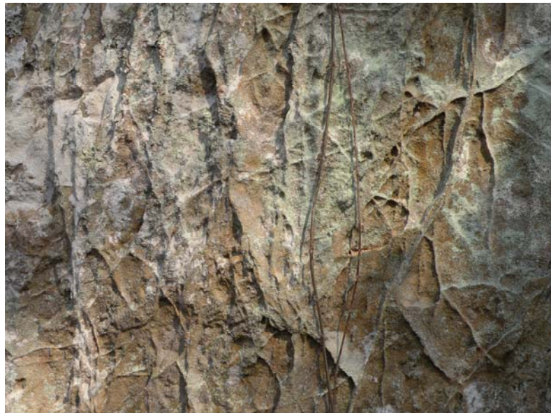
Figure 12. Deformation bands in block of "middle Bloyd sandstone".
