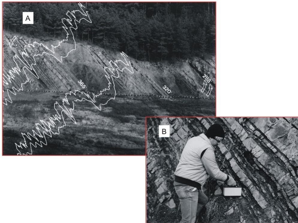
Figure 10: Outcrop gamma ray profiling using a hand-held scintillometer (geiger counter). A. shows two sets of logs (white lines) over a part of the DeGray Spillway section. B. shows the scintillometer being held against the rock so that the gamma-ray counts can be measured. Figures from Jordan et al., 1993.
