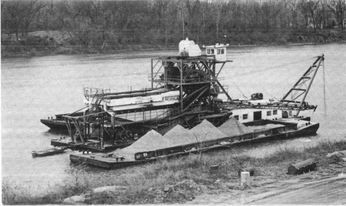
Figure 5 - Stop 1. Sand dredge and barge operated by the Arkansas Sand Company on the Arkansas River at the abandoned Big Rock quarry in North Little Rock.
