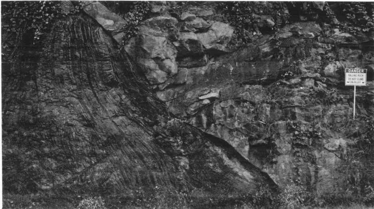
Figure 33 - Stop 16. A fairly clean sandstone of an upper submarine fan channel (right) incised in shale and siltstone of the fan lobe (interchannel) or slope facies (left), at the top of the lower Atoka Formation at Blue Mountain Dam.
