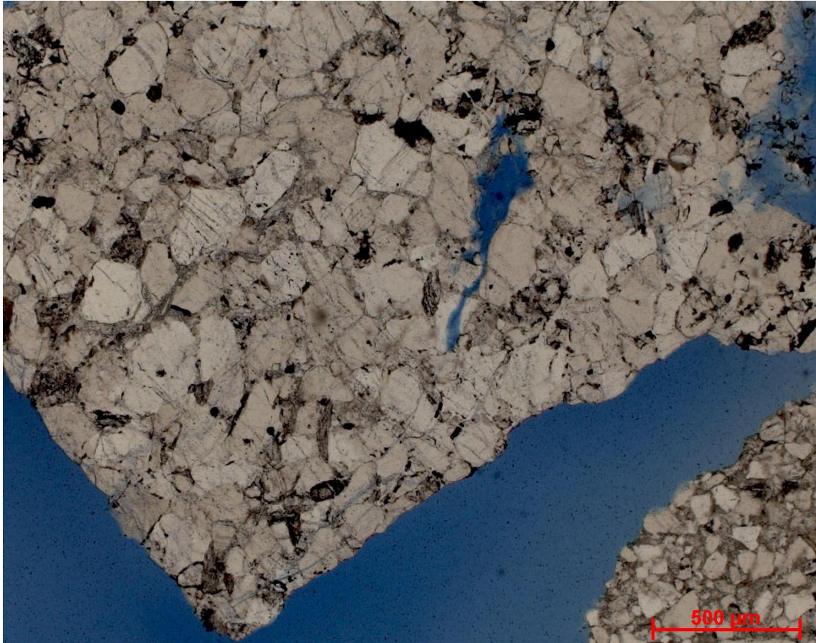
Figure 3. Photomicrograph of thin section of well cuttings in the Mississippian Stanley Formation at 7,240-50 ft (2,207-10 m) (plane polarization). Highly compacted fine- to medium- and medium- to coarse-grained sandstones. Moderate quartz overgrowth and calcite cementation. Mica (?) in the ground mass with high birefringence.
