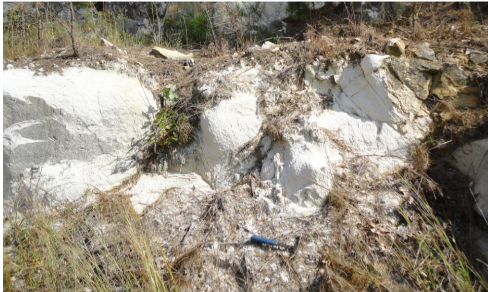
Figure 3f. Almost completely weathered sandstone: Hartshorne Sandstone at Cove Mountain and AR Hwy. 247 approximately 3.6 miles south of Pontoon.
