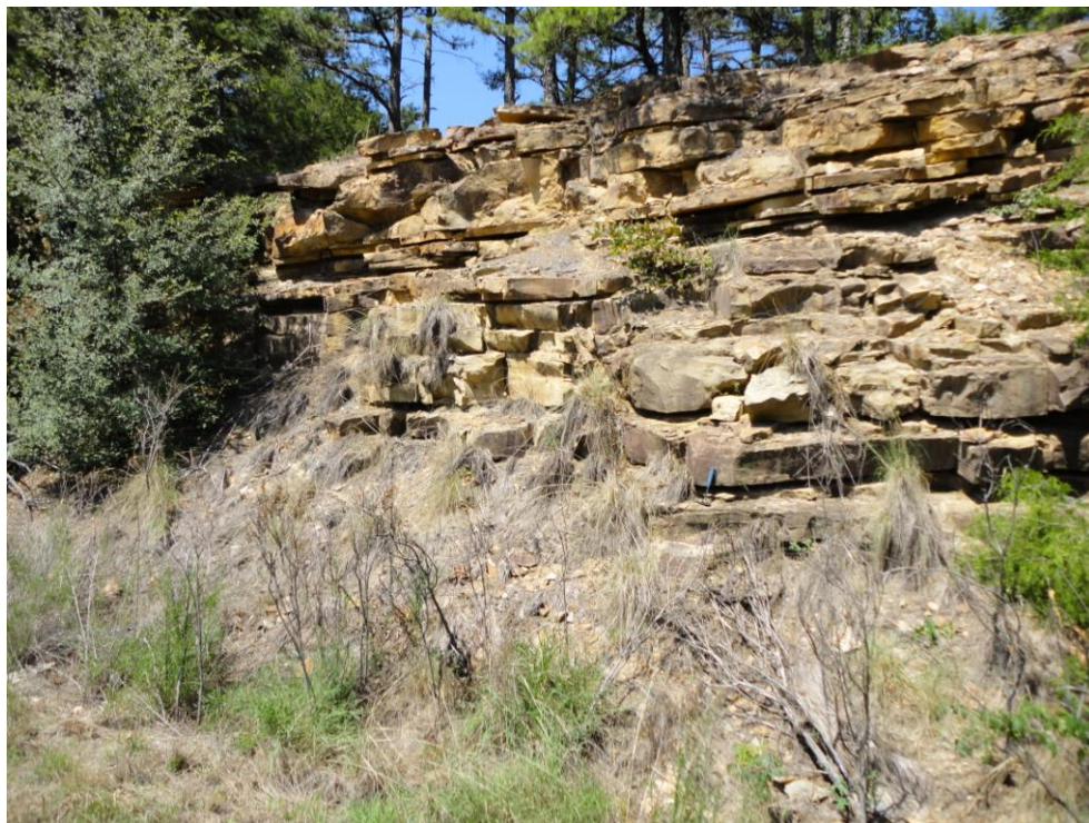
Figure 3c. Moderately weathered sandstone: Hartshorne Sandstone on I-40 approximately one-half mile east of Interchange #74 at London.
