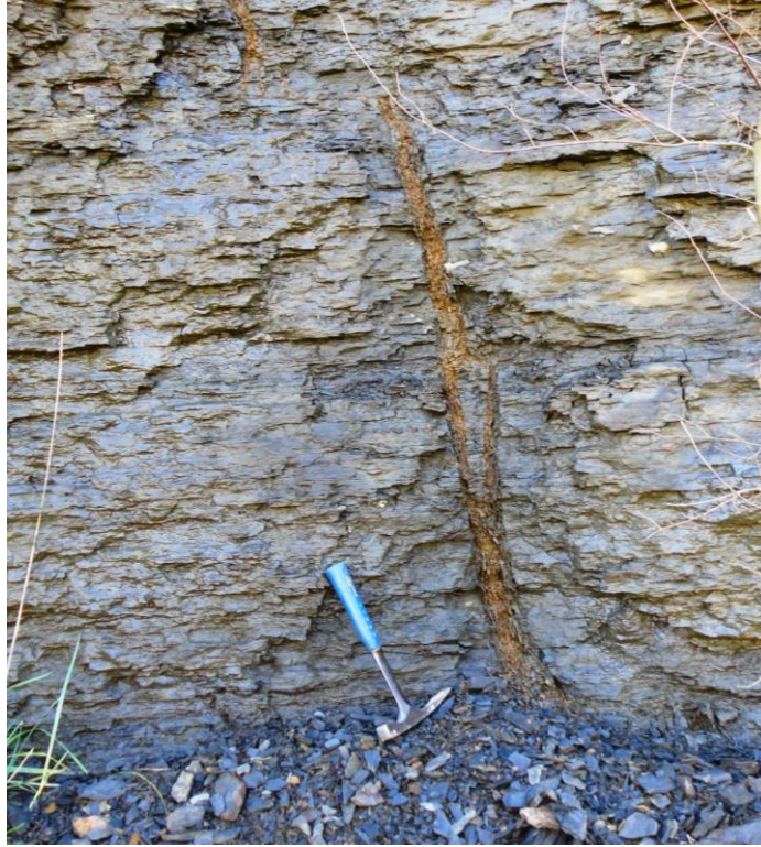
Figure 4e. Heavily weathered joint plane in shale: Atoka Formation along AR Hwy. 22 nearly two miles west of Dardanelle, Arkansas. The photograph illustrates development of platy shale fragments aligned along the joint plane.
