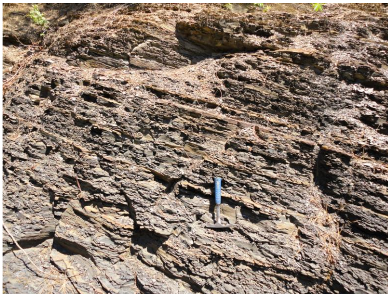
Figure 4b. Moderately weathered shale: McAlester Formation at the spillway of Horsehead Lake approximately 2.7 miles north of Hunt on AR Hwy. 164.
