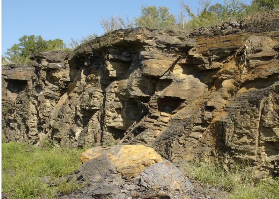
Figure 4c. Moderately weathered shale: Atoka Formation along AR Hwy.7 nearly two miles north of the I-40 Interchange #81 at Russellville.
