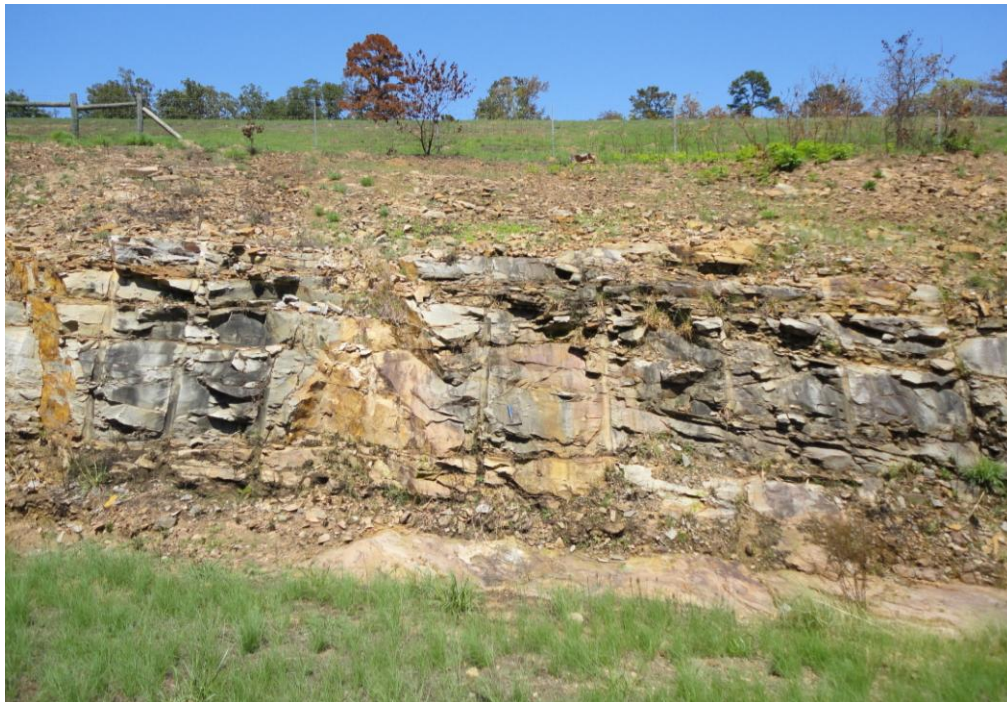
Figure 3b. Slightly weathered sandstone: Hartshorne Sandstone at the I-40 Interchange #78 west of Russellville.
