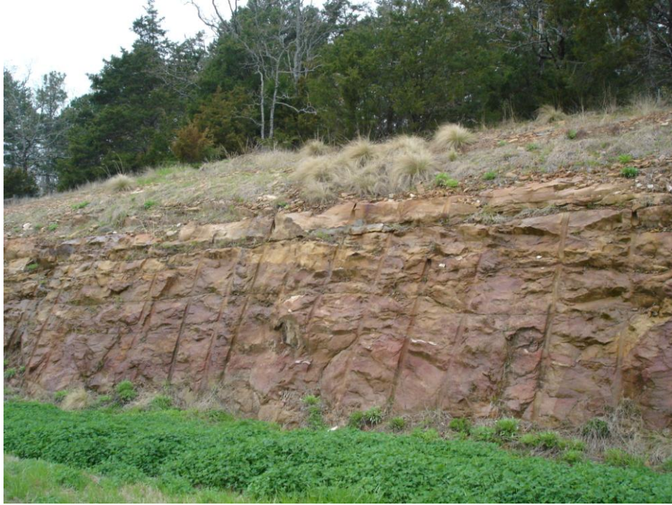
Figure 3a. Unweathered sandstone: Hartshorne Sandstone at the I-40 Interchange #78 west of Russellville.
