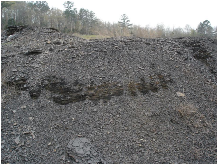
Figure 4d. Heavily weathered shale: McAlester Formation at Robertsons Lane off US Hwy. 64 nearly two miles west of I-40 Interchange #78 west of Russellville.
