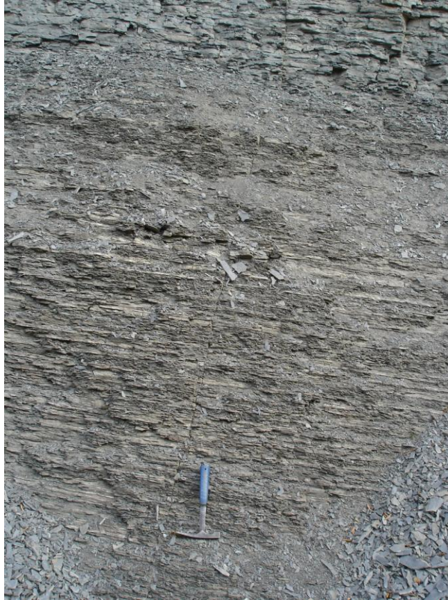
Figure 4a. Unweathered to slightly weathered shale: Atoka Formation along AR Hwy. 9 roughly 1.75 miles south of I40 Interchange #108 at Morrilton.
