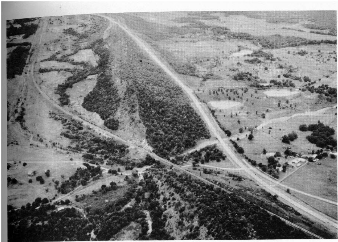
Fig. 14. -- Aerial view southwest along Limestone Ridge with Limestone Gap in the foreground. Stop 3 is in cutbanks along United States Highway 69. The trace of the Katy Club fault is between the ridge and the railroad. The Choctaw fault is to the right of the ridge. Both strike southwest and dip southeast, probably sharing the dip of the Wapanucka limestone in the ridge which is 42 degrees to the left. (Photograph courtesy Magnolia Petroleum Company)
