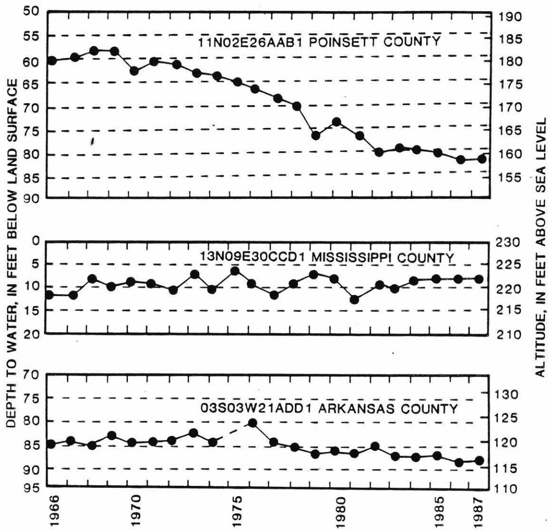
Figure 3. sheet 1 of 2.--Water-level hydrographs for selected wells completed in Quaternary deposits.
