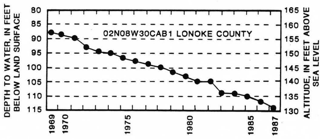
Figure 3. sheet 2 of 2.--Water-level hydrograph for selected wells completed in Quaternary deposits.
