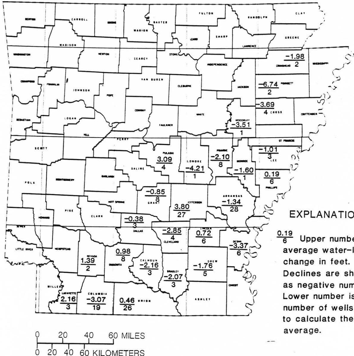
Figure 2.--Average water-level changes by county between 1982 and 1987 of wells completed in the Sparta and Memphis Sands.
