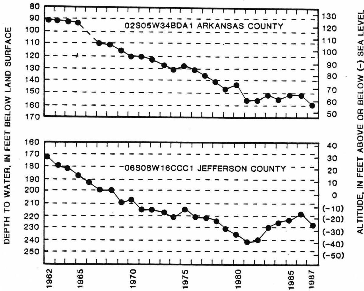
Figure 4. sheet 1 of 2.--Water-level hydrographs for selected wells completed in the Sparta Sand.
