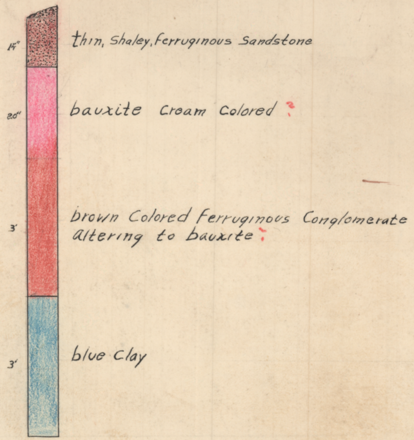
Columnar Section in Test Shaft 2
