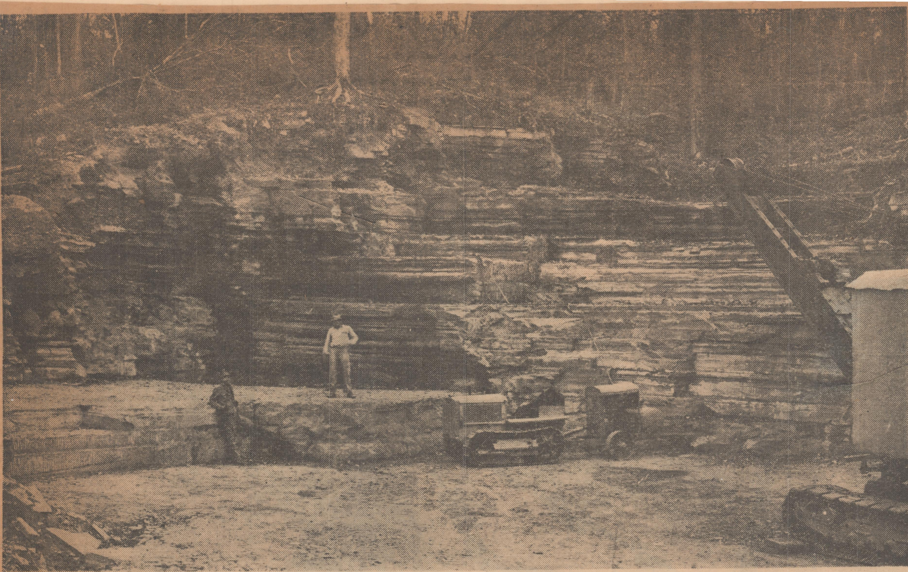
Black marble quarry near Batesville. Holes are drilled in rock outlining block to be removed. Wedges driven into the drill holes force block out of position. (Photographs by courtesy of Esso Oilways.)
